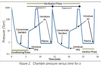
hydrogen peroxide gas plasma sterilization cycle.
