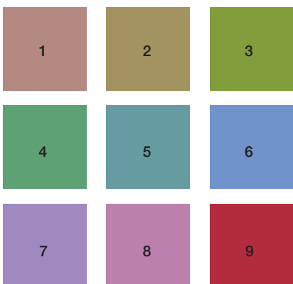
Figure 3. Color Rendering Indices: CRI is the average of the first eight pastel color rendering indices. The special color rendering index for the 9th color sample, R_9 , is not included in the average, but is very important to surgeons because it represents the ability of a light source to render deep, saturated red.
